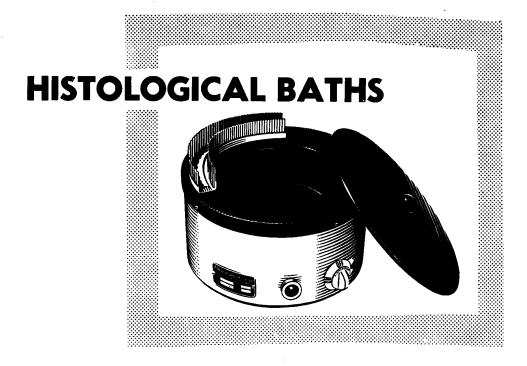
A range of Paraffin Section Mounting Baths indispensable in the modern Histological Laboratory. Uniform controlled heating provides constant temperature on the water surface; air bubbles are eliminated. Sections are clearly visible against the matt black background. Models with built-in energy regulators or thermostats can be supplied.
