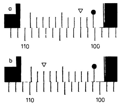
Photographs of a Vernier scale on a microscope stage in two different positions, (a) showing a reading of 100.2 mm (arrowhead), and (b) showing a reading of 100.8 mm (arrowhead). The difference between the two readings is therefore 0.6 mm.
