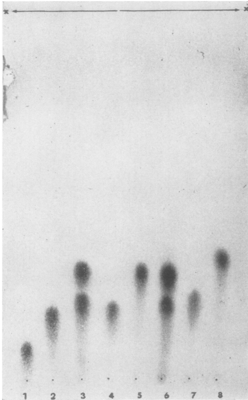
FIG. 4 Thin-layer chromatogram of sugars on a 20 × 10 cm. plate (procedure as in text).
