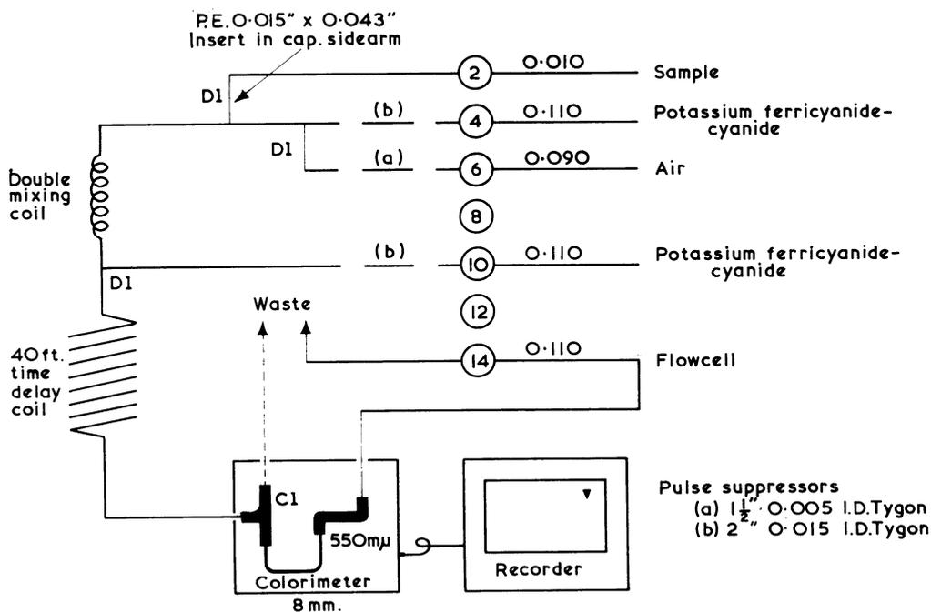
FIG. 1. Flow diagram for haemoglobin estimation.
