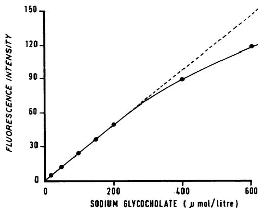
Fig. 1 Calibration curve for sodium glycocholate showing relationship between intensity of fluorescence (in galvanometer units) and concentration of standard solutions.
