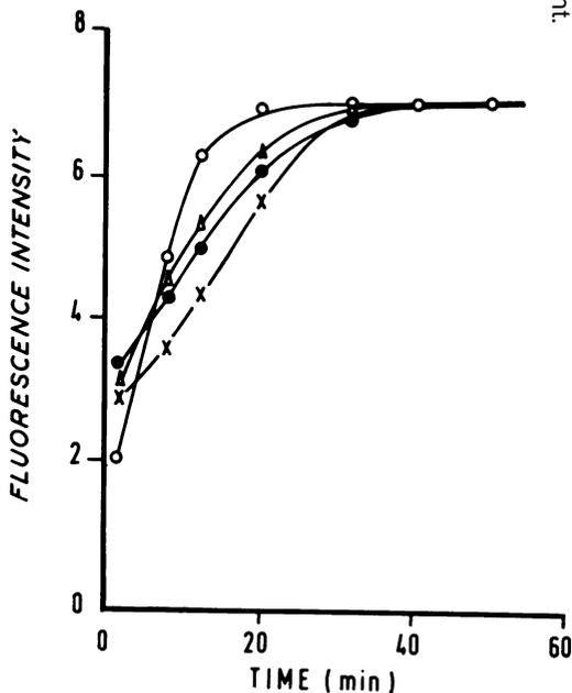
Fig. 3 Development of fluorescence in reaction mixtures containing 50  $\mu\text{l}$  bile salt solutions (24  $\mu\text{mol/litre}$ ) at 37°C in relation to time
