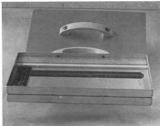
each corner of side B. These holes are used for drainage. The lid is made of aluminium sheet  $8\frac{1}{2}$  in  $\times$   $4\frac{1}{2}$  in with the handle centrally placed. The tray can hold eight slides.
