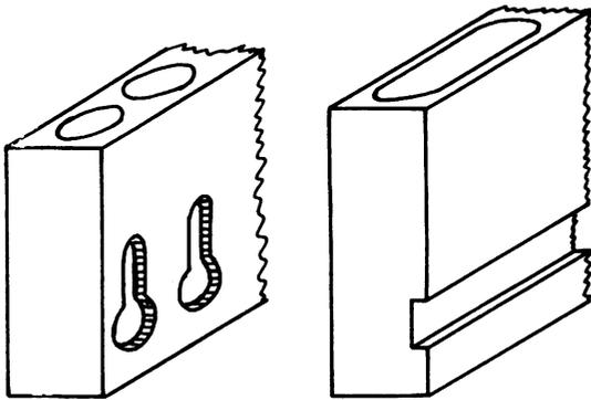
Figure Diagram of segment of standard LKB sample rack (left) and modified rack (right). Note the extra height, longitudinal groove, and reagent cavity of the modified rack.
