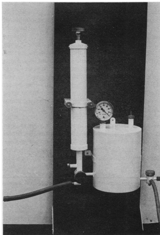
Fig 1 Photograph of carbon dioxide dosage system.
