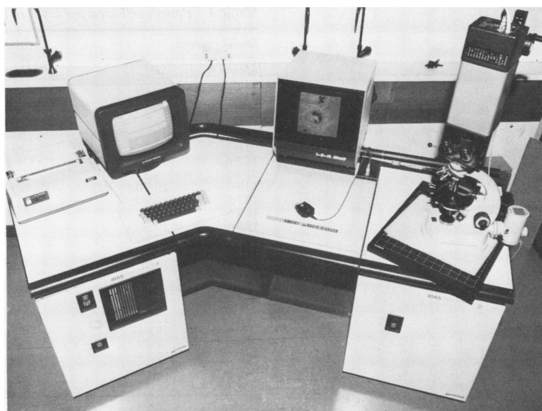
Fig. 1 General view of the IBAS 2 Image Analyser prepared for Paneth cell area measurement. The central monitor shows the Paneth cell image that has been obtained from a slide under the microscope on the right of the picture.
