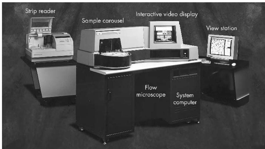
**Figure 1** The IRIS 939Udx instrument, optional strip reader, and view station.
