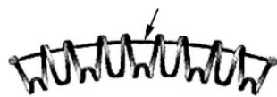
Figure 6 Gianturco-Roubin II by Cook Inc. The longitudinal strut is indicated by a black arrow. Original image taken from website ( http://www.cis.tugraz.at/biomech/Proj1.htm ).
