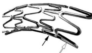
Figure 5 Express (TAXUS Express 2 ) by Boston Scientific. Micro elements (black arrow) and Macro elements (white arrow) are indicated. Original image taken from TAXUS Express 2 pamphlet.
