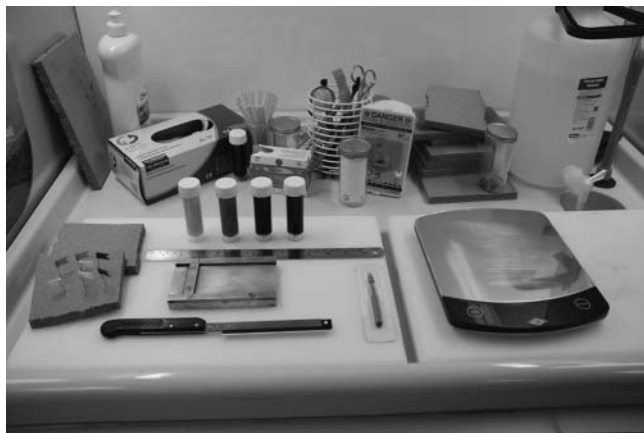
Figure 1 The basic kit required for sampling, including cutting guide plate, scales, knife, cork board, punch biopsy and a ruler. This figure is only reproduced in colour in the online version.
