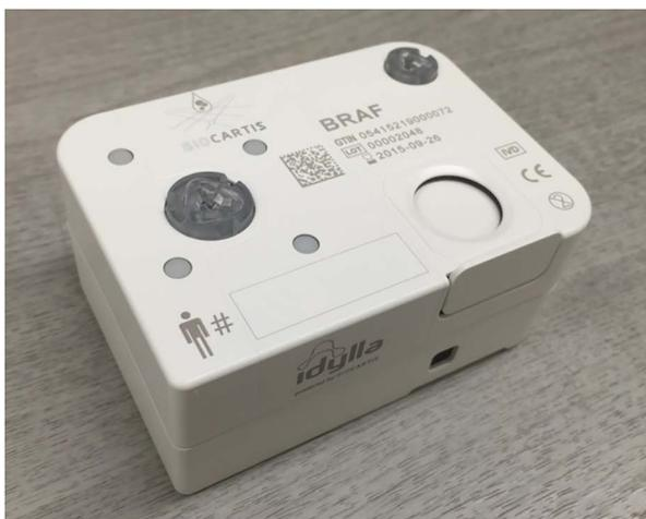
**Figure 3** The Idylla *BRAF* Mutation Test cartridge (95×70×40 mm).
