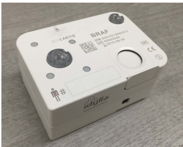
Figure 3 The Idylla BRAF Mutation Test cartridge (95×70×40 mm).
